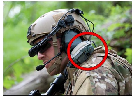
Figure 8. QinetiQ EARS shoulder mounted sensor [7].
