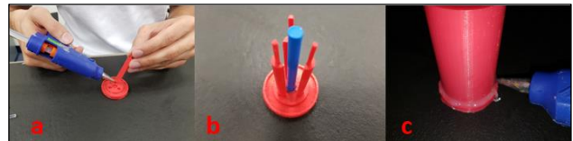
Figure 3. a) put hot glue on the holes, b) pneumatic template, and central channel template molds are placed on the base mold, and c) the threaded container, entire mold was assembled with hot glue.
