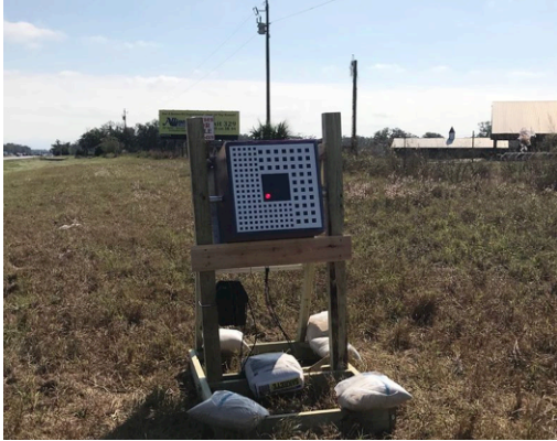
Figure 2. Prototype of sensor during a live field test in winter of 2017 along I-75 near Wildwood, FL.
