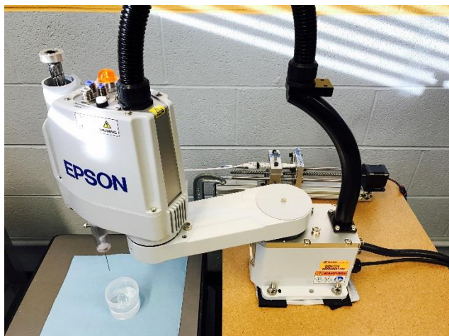
Figure 1. Robotic soft matter 3D printing system setup.
