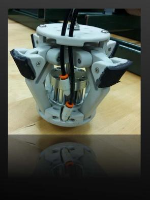
The current grippers are able to provide a maximum gripping force of ~40 lbs
