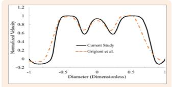
**Figure 3:** Validation of the computational methods by comparing the velocity distribution in the current study with a previous experimental study [20].
