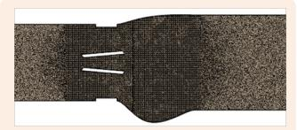
Figure 2: High quality mesh generated in the flow domain especially close to the leaflets and aortic sinuses.
