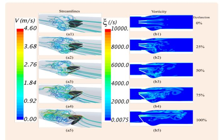
Figure 4: Flow field around the valve
