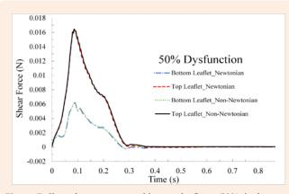
**Figure 7:** Shear forces on top and bottom leaflet at 50% dysfunction for Newtonian and non-Newtonian flows.
