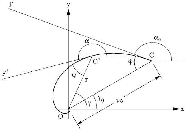
Fig. 10 A counterclockwise logarithmic spiral motion of C
