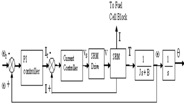
Fig. 9. Full Detail Diagram of SRM Drive Control
