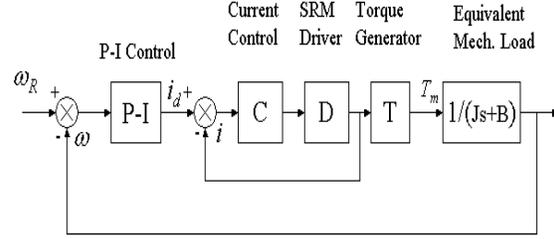
Fig. 1. Block Diagram of SRM Drive Speed Control
