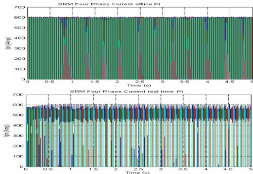
Fig. 14. Off-Line and Real-Time Simulation of SRM Current
