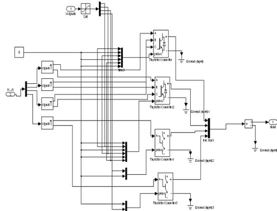
Fig. 7. Simulation Diagram for Current Converter
