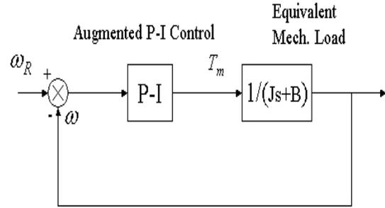
Fig. 5. Block Diagram for Augmented  $P-I$  Control Design
