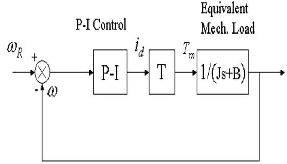
Fig. 4. Block Diagram for  $P-I$  Control Design
