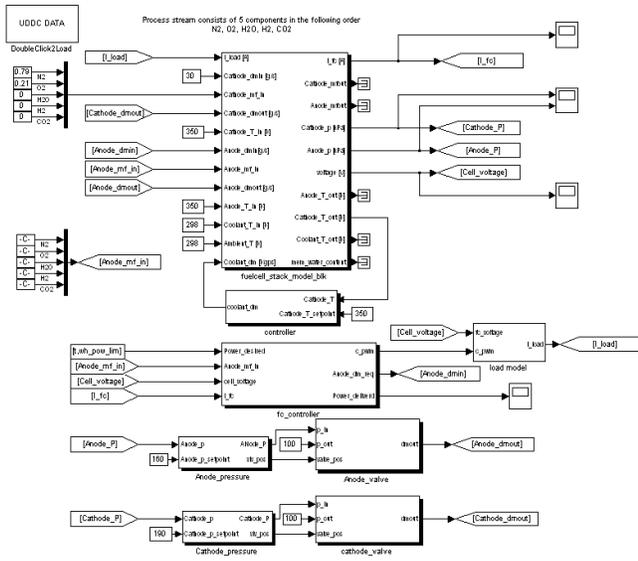
Fig. 6. Block Diagram of Fuel Cell Stack
