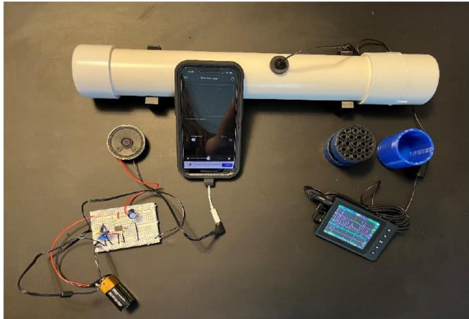
Low-Cost Impedance Tube Fixed end configuration
